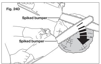
When bucking on a slope, always stand on the uphill side of the log. When cutting through the log, maintain control by releasing the cutting pressure near the end of the cut without relaxing your grip on the chain saw handles. Do not let the chain contact the ground.
