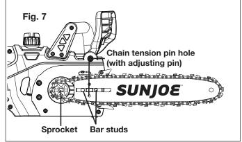
7. Adjust the chain tension as needed by adjusting the chain tensioner screw with the supplied flat-tip blade screwdriver. Make sure to align the chain tensioner screw with the pin hole (Fig. 8).
