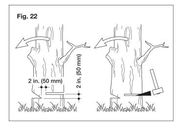
Make the lower horizontal notching cut first.
