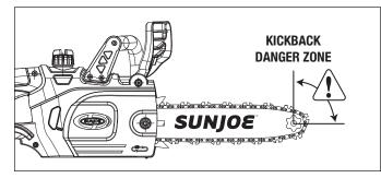
**WARNING!** Kickback may occur when the nose or tip of the guide bar touches an object, or when the wood closes in and pinches the saw chain in the cut.
